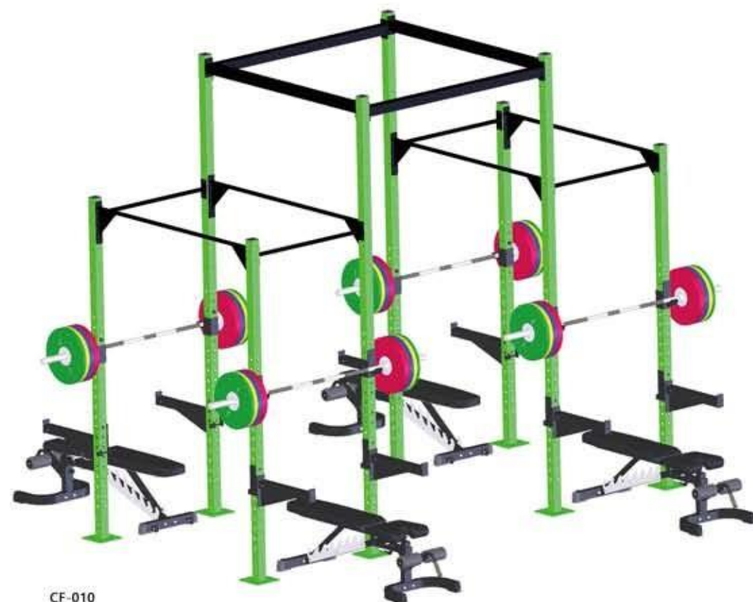
CF-010 Free Standing RIG Model Size:4'-6'-4' Main tube:75*75*3mm,Monkey bar:Φ32*5mm Height:2.75m-3.6m,Depth:1.2m,Length:4.2m Color:Black matte/Green smooth
